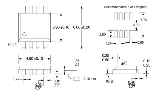
Refer to JEDEC MS-012 for complete dimensions and notes. All dimensions in <u>millimeters</u>.
