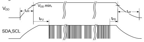
**Power Cycle Timing** ( $T_A = -40$ °C to +85°C,  $V_{DD} = 4.5$ V to 5.5V unless otherwise specified)
