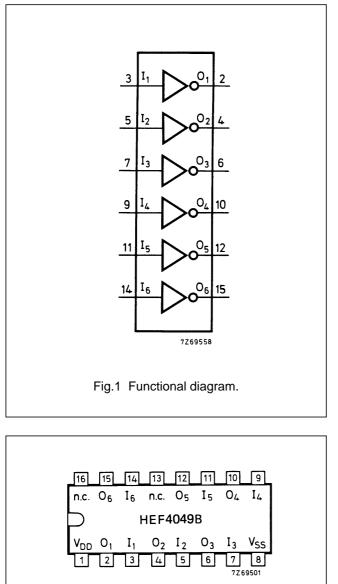
Fig.2 Pinning diagram.
