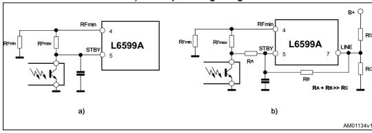
Figure 24. Burst mode implementation: a) narrow input voltage range; b) wide input voltage range
