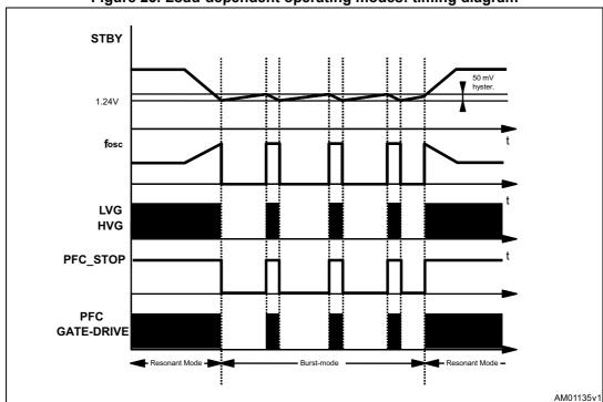
Figure 25. Load-dependent operating modes: timing diagram
