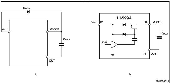
The diode prevents any current being able to flow from the VBOOT pin back to Vcc, in case the supply is quickly turned off when the internal capacitor of the pump is not fully discharged. To drive the synchronous DMOS a voltage higher than the supply voltage Vcc is necessary. This voltage is obtained by means of an internal charge pump (*Figure 31*b).
