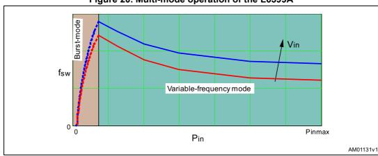
Figure 20. Multi-mode operation of the L6599A
