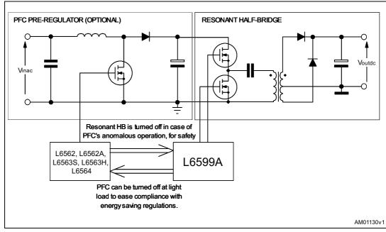
Figure 21. Typical system block diagram
