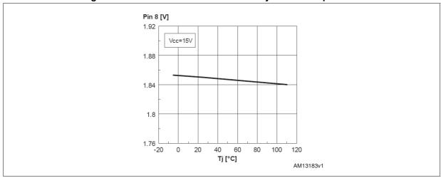
Figure 19. Latched disable threshold vs. junction temperature
