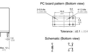
Dimension: Less than 1mm .039inch: Min. 1mm .039inch less than 3mm .118 inch:  $\pm 0.2 \pm .008$ Min. 3mm .118 inch:
