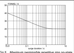
Fig.5. Maximum permissible repetitive rms on-state current  $I_{T(RMS)}$ , versus surge duration, for sinusoidal currents, f = 50 Hz;  $T_{mb} \le 103$  °C.
