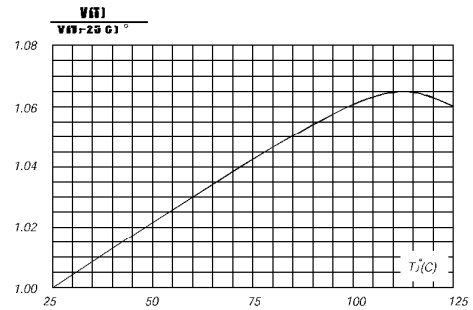
FIG.2-Relative variation of V0 versus junction temperature (typical values)
