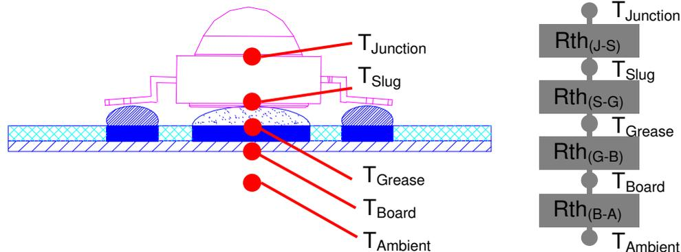
$$R_{th(J-A)} = R_{th(J-S)} + R_{th(S-G)} + R_{th(G-B)} + R_{th(B-A)}$$
