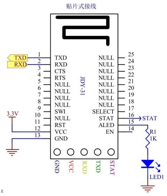
patch application: general application only need to connect VCC, GND, RXD, TXD 4 pins, if you need to actively disconnect in the connection state, send AT+DISC in the connection state
