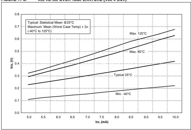
FIGURE 11-9: Vol vs. Iol OVER TEMPERATURE (VDD = 5.0V)
