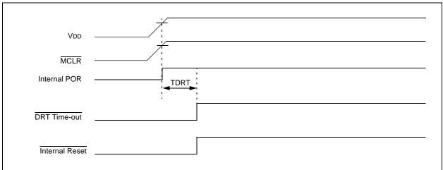
TIME-OUT SEQUENCE ON POWER-UP (MCLR TIED TO VDD): SLOW VDD RISE FIGURE 8-5: TIME
