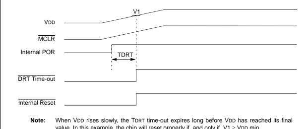
value. In this example, the chip will reset properly if, and only if, V1 ≥ VDD min.
