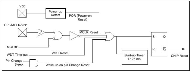
FIGURE 8-3: TIME-OUT SEQUENCE ON POWER-UP (MCLR PULLED LOW)
