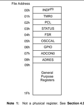
Note 1: Not a physical register. See Section 4.9 "Indirect Data Addressing; INDF and FSR Registers".
