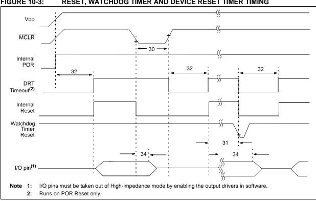
**FIGURE 10-3:** RESET, WATCHDOG TIMER AND DEVICE RESET TIMER TIMING
