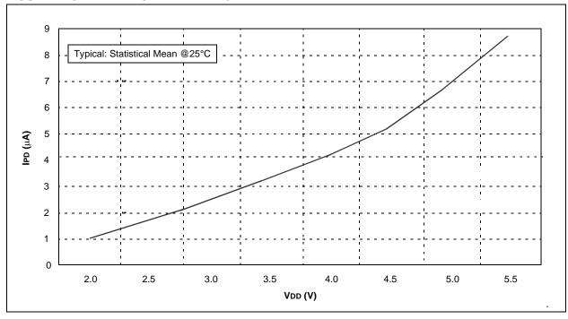
FIGURE 11-6: MAXIMUM WDT IPD vs. VDD OVER TEMPERATURE
