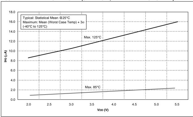
FIGURE 11-5: TYPICAL WDT IPD vs. VDD
