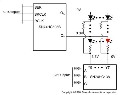
Figure 4. LED Matrix Driver Application
